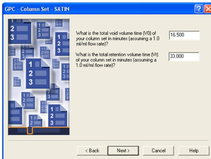
Figure 3-11 Setting  $V_0$  and  $V_t$  Values
