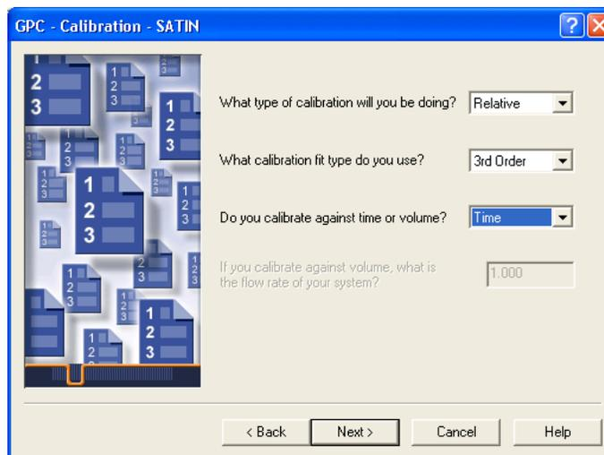
Figure 3-10 Setting GPC Calibration Parameters
