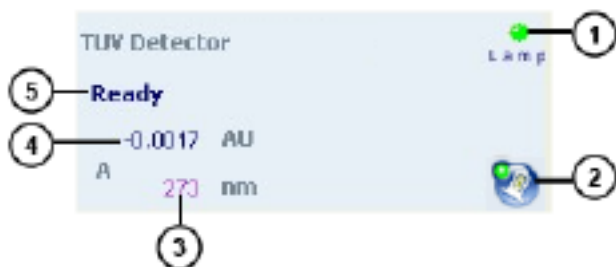
Figure 3–10: TUV detector control panel
