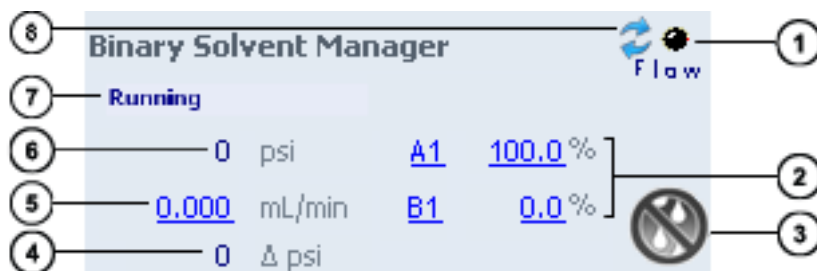
Figure 3–2: BSM control panel
