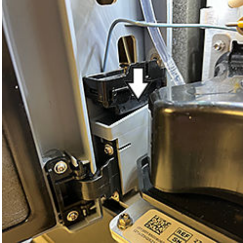
Figure 4–18: Installing the drain cup
