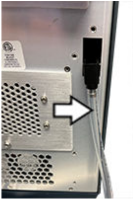
Figure 4–22: Disconnecting condensate waste line
