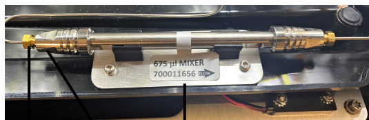
Figure 8–7: Location of the inlet compression fitting for the mixer
