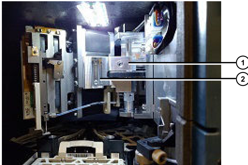
Figure 8–44: Magnet location in needle carriage arm
